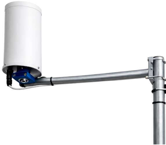
Figure 43 Rain gauge connected to the bracket on top of the pole
