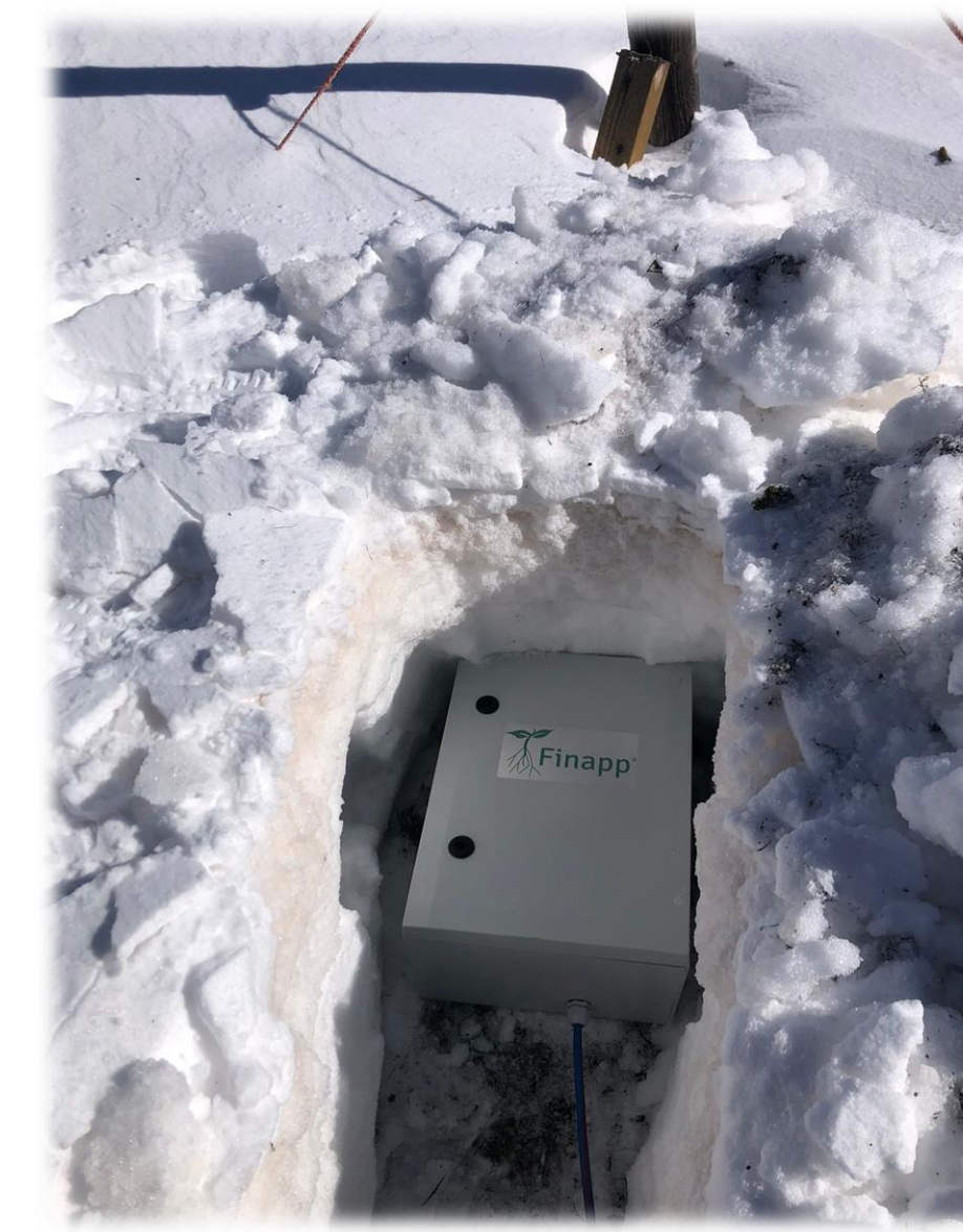
"On-ground" probe for Local SWE measurements
