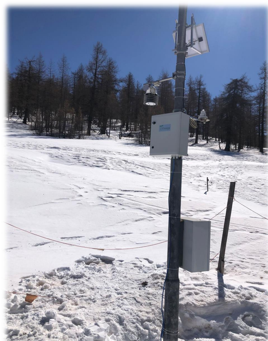
"On-air" probe for Areal SWE measurements
