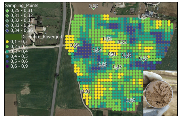
Fig. 6: Comparison between soil moisture map obtained by CRNS-Rover and gravimetric soil moisture in different sampling points within the field.
