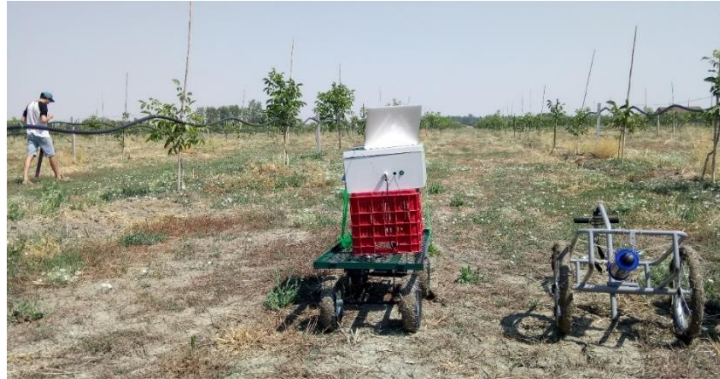
Figure 1. Experimental instrument setup with, starting from the left of the photo: portable TDR in the hands of the operator, CRNS, and GRS probes mounted on wheels
