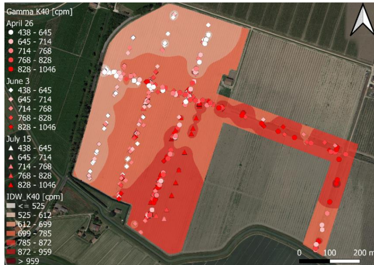
Figure 5. K-40 counts acquired by the gSMS during different days of surveys and data interpolation.
