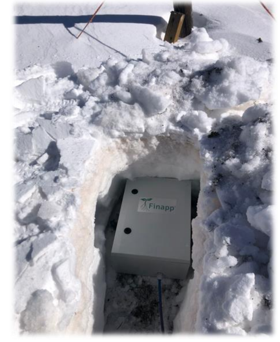
"On-ground" probe for Local SWE measurements
