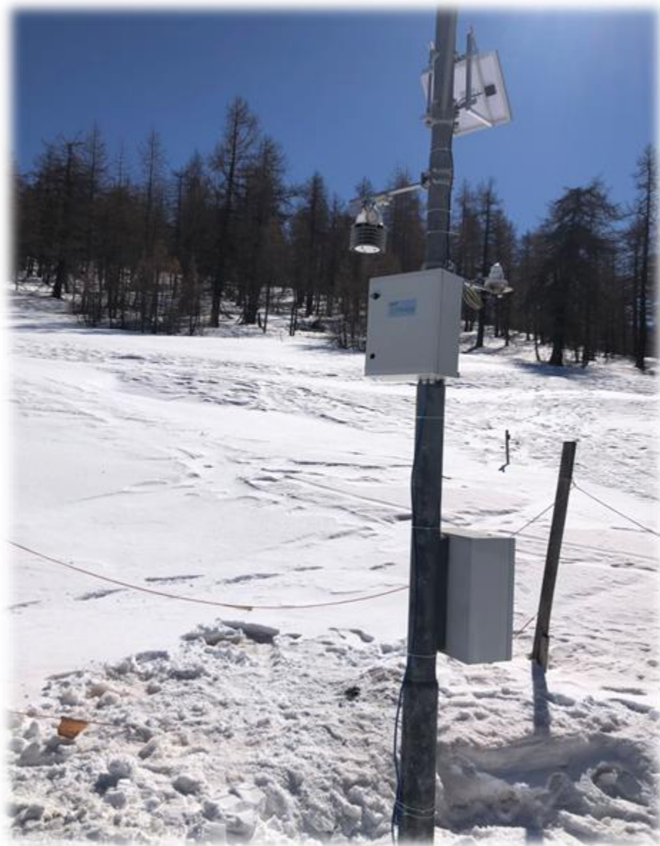
"On-air" probe for Areal SWE measurements
